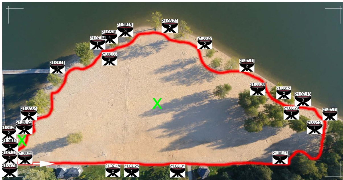
137 — route (≈ 412 m) for the trolley with the installed measuring equipment ☞ - location of barbecue facilities X - sampling points for petrographic tests
