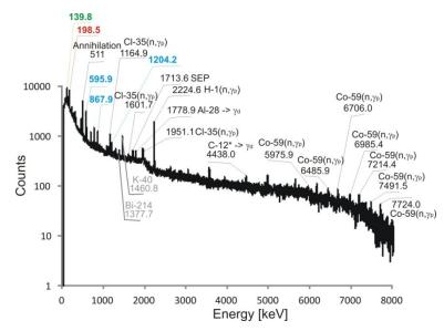
The spectrum measured with HPGe detector in the operator room during emission of 18 MV beam from Elekta. The peaks related to neutron reactions occurring in the Ge crystal in the detector HPGe and some others are marked.
