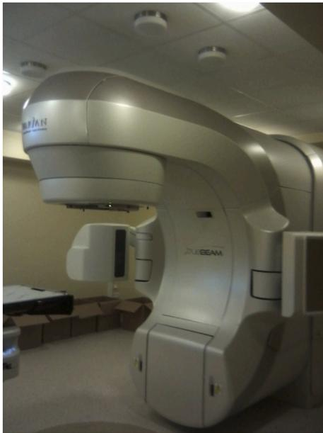
Fig. 2. The TrueBeam linear accelerator by Varian used for irradiation of CIEDs.
