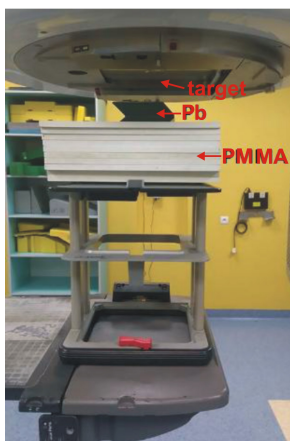
Fig. 1. A target located on the accelerator window and the lead-PMMA system.
