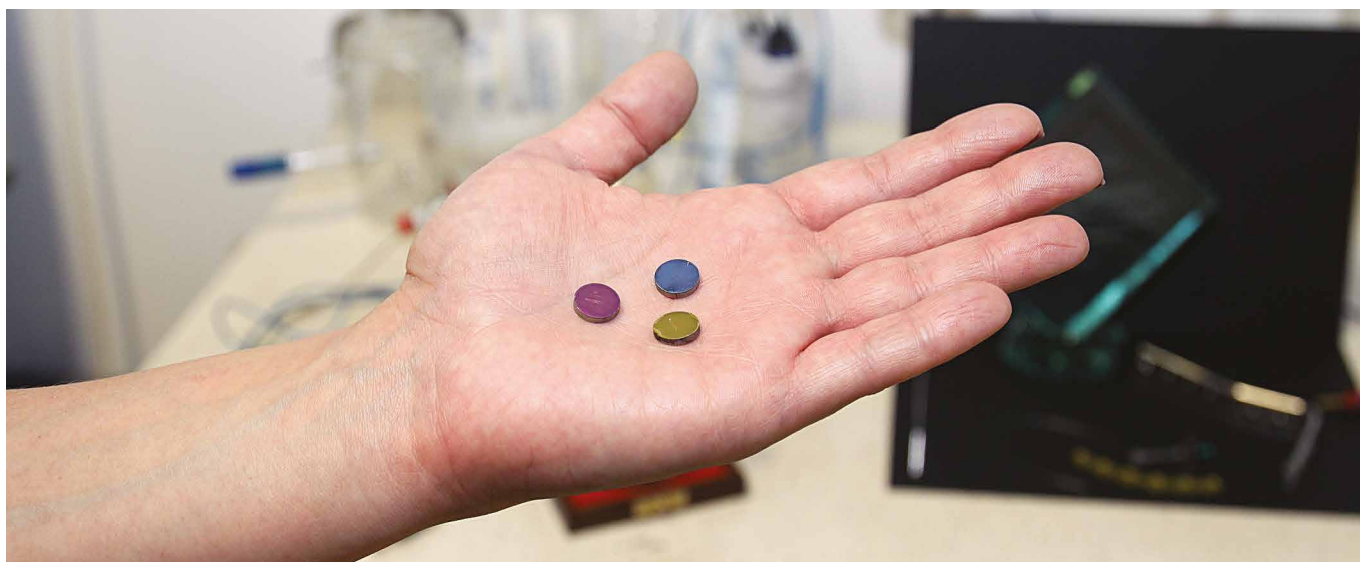
Implant alloy samples of Ti15Mo with hybrid coatings deposited in various electro-chemical conditions / Photo. Małgorzata Kłoskowicz
