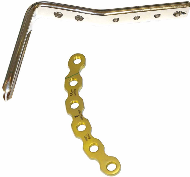
Scientists from the Institute of Materials Engineering of the University of Silesia work on modifications of biomaterial surfaces, mainly titanium alloys, in order to improve their corrosion resistance and thus to enhance their biocompatibility / Photo. Agnieszka Sikora
